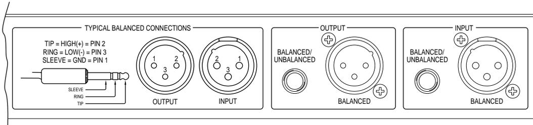
Figure 8 - View of rear panel connectors.
