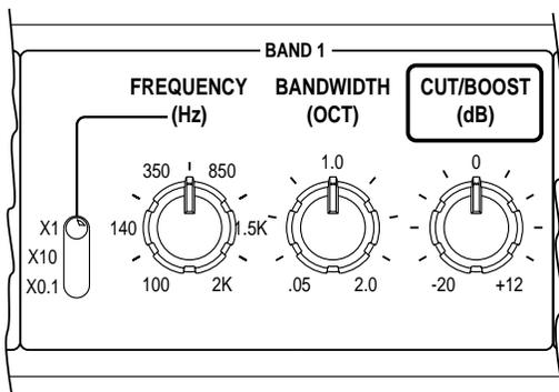
Figure 4 - Front panel view of one EQ band.
