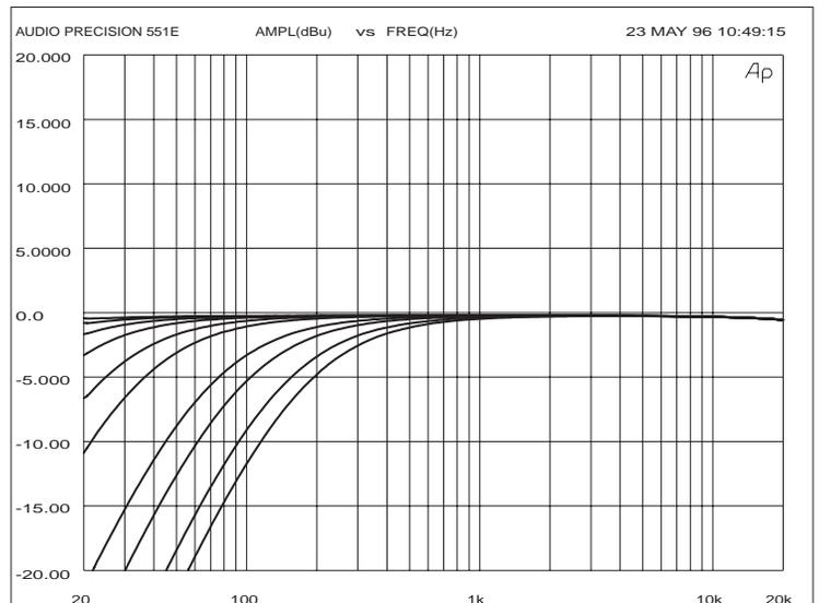
Diagram 2 - Low cut filter with 12 dB per octave.
