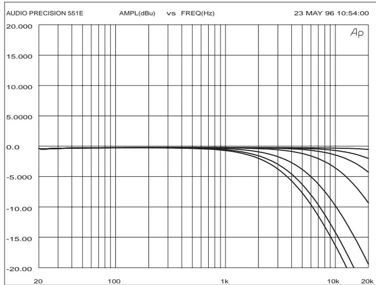
Diagram 3 - High cut filter with 12 dB per octave.
