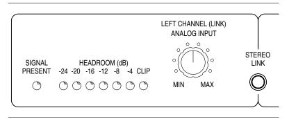
This section contains the analog input controls for the left and right analog inputs.
