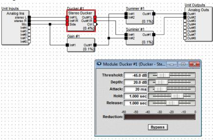
In SymNet Composer, using a ducker has been greatly simplified. The Ducker module has built in side-chain mix controls. By default, the side-chain input is muted. To mix the side-chain signal back into the program audio, simply turn off the mute and adjust the level for which the side-chain should be mixed into the program audio.
