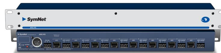
The ARC-PS is a hub with 8 ARC ports that is handy for providing data and power to many ARCs. To use with Jupiter, simply wire one end of a CAT-5 cable to the 3 pin RS-485 terminal on the back of the ARC-PS. A = pin 4, B = pin 5, Ground = pin 6. Keep the RJ-45 end of the CAT-5 intact for connection to the Jupiter ARC port. No further configuration is required and the network of ARCs will now be available for programming in the Jupiter software.
