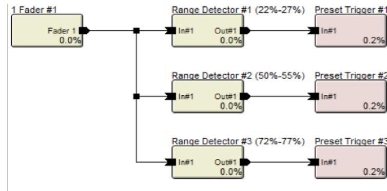
The problem occurs when making a selection on the multi-position switch, for a brief moment the voltage may bounce to 0% or 100%, causing the other presets in between the desired setting and the bounce to trigger unexpectedly.
