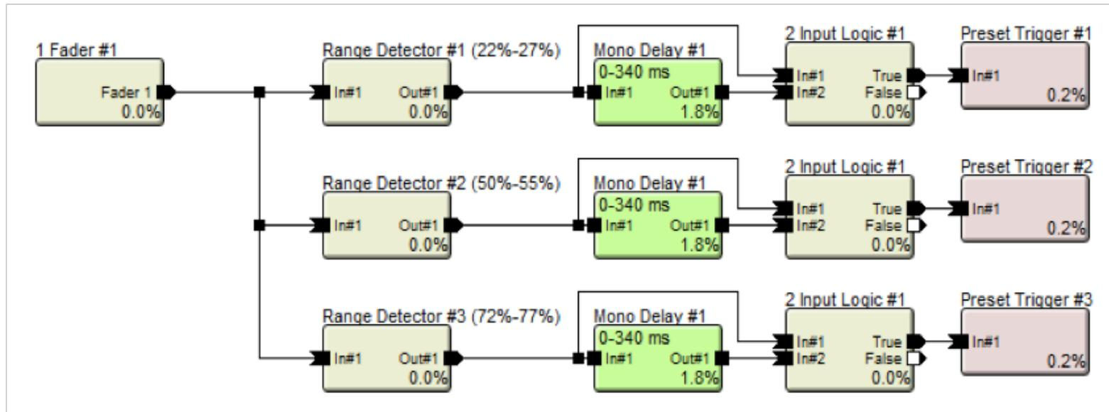
The delay time sets how long the control signal must be settled and consistent before triggering the preset. A default setting of 100 ms is suggested. As long as the switch bounce settles before 100 ms, the bounce will not register and trigger unintended presets.
