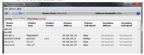
Step 4: Double Click on the "Device Name" of the SymNet unit to open the "Device View".
