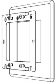
**1b.** Optional trim ring installation: Holding the T-5 trim ring in place, screw the universal flush mount bracket into the wall mounted back box with the three holes positioned at the top.
