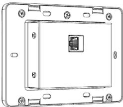
**3** Snap the T-5 or T-5 Gen 2 Touchscreen onto the universal flush mount bracket.
