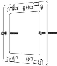
**1a.** Screw the universal flush mount bracket into the wall mounted back box. \*Note proper flush mount bracket orientation, with the three holes positioned on the top.
