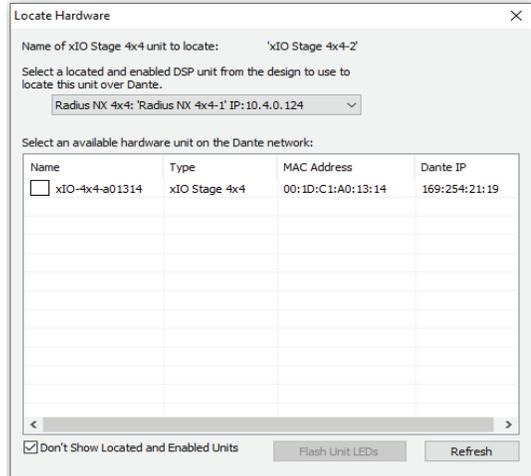
The Locate Hardware dialog will scan the selected Radius NX, Prism or Edge unit and list the xIO Stage 4x4 unit. Select the physical xIO Stage 4x4 unit you wish to use and click the Select Hardware Unit button.
