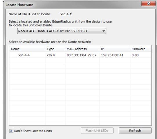
The Locate Hardware dialog will scan the selected Radius, Prism, or Edge unit and list xIn 4, xOut 4, and xIO 4x4 units. Select the physical xIn 4, xOut 4, or xIO 4x4 unit you wish to use and click the Select Hardware Unit button.
